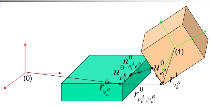
$$\begin{split} \text{Kinematic constraint:} \quad & d_s^E \left( e_i^A, e_j^B \right) = 0 \\ \text{The Euclidean distance is computed as:} \quad & d_s^E \left( e_i^A, e_j^B \right) = (n_{e_i^A e_j^B}^0)^t \left( r_{v_k^A, v_n^B}^0 \right) \\ & = (\frac{1}{\left\| \widetilde{u}_{e_i^A}^0 u_{e_i^B}^0 \right\|^2} \widetilde{u}_{e_i^A}^0 u_{e_j^B}^0)^t \left( r_1^0 + R_1^0 r_{v_k^A}^1 - r_{v_n^B}^0 \right) \end{split}$$
